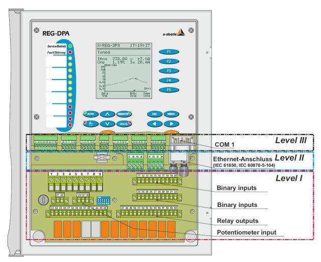
Figure 11: Location of the connector terminals
