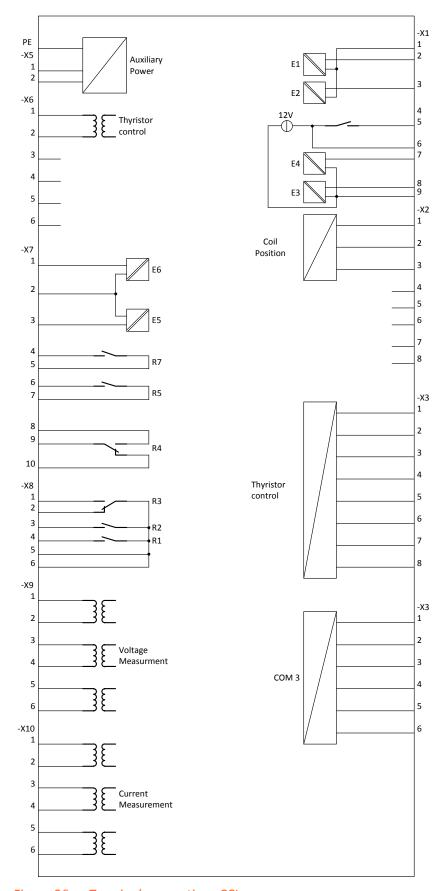
Figure 26: Terminal connections CCI
