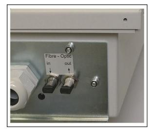
Figure 9: Fiber optic (ST-connection)
