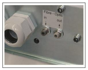
Figure 10: Fibre optic (FSMA-connection)
