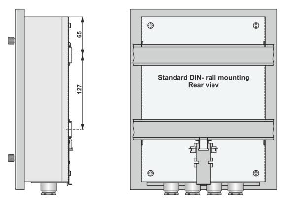
Figure 15: Mechanical dimensions, standard DIN-rail assembling
