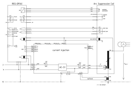
Figure 22: Uo measurement over external or remote voltage transducer
