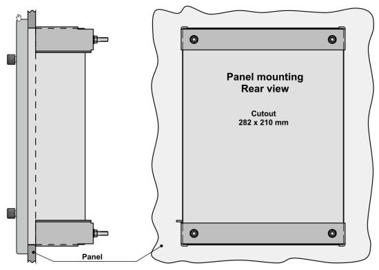
Figure 14: Mechanical dimensions, Panel mount housing
