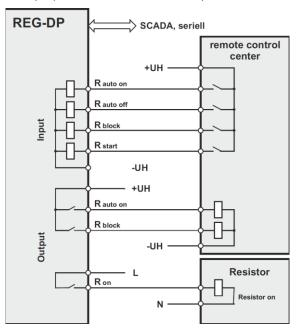
Figure 5: Example for the resistor control
