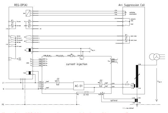
Figure 21: REG-DPA connection, current injection and Petersen coil;
