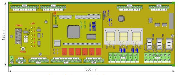
Figure 25: Dimensions of current feed-in controller (CCI)
