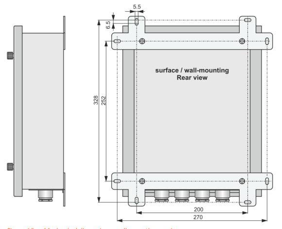
Figure 16: Mechanical dimensions, wall-mounting version
